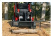
**COMPACT FOOTPRINT** The narrow model is just 33.7" (86 cm) wide and fits through standard 36" gates. At just 41" (104 cm) wide, the wide-track model is also easy to maneuver.
