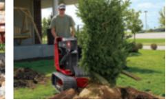
**TREE FORK** Hydraulic fork arm opens to handle large trees and shrubs. Angle design allows for gentle handling. Opening at tip: 25"
