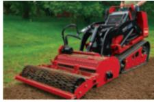
**SOIL CULTIVATOR** Bury stones, soil clods, debris and grass. Prepares seed bed in one pass, tilling soil up to 5.5" deep. Adjustable grading bar and comb teeth leave perfect germination environment. Working width: 36"
