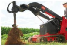
HIGH-TORQUE AUGER POWER HEAD Designed specifically to power up to 30" diameter augers in the toughest soil conditions. Auger bits from 6" to 30". Max bit speed: 70 rpm @ 14.3 gpm Bit length: 42"; 12" and 24" extensions available Torque: 1,514 ft-lbs @ 3,000 psi
