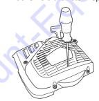
Lubricate the recoil spring with light oil. Fit the pulley and tension the recoil spring.
