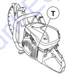
Rec. idle speed: 2700 rpm
