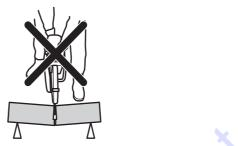
If the blade is pinched or stalled in the kickback zone, the reactive force will push the power cutter up and back towards the user in a rotating motion causing serious or even fatal injury.
