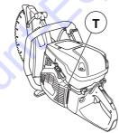
Rec. idle speed: 2700 rpm
