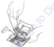
• Remove any remnants of the old starter cord and check that the return spring works. Insert the new starter cord through the hole in the starter housing and in the cord pulley.
