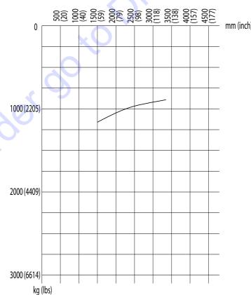
1. On outriggers – forward DXR270 - weight on ground will appear on two outriggers.
