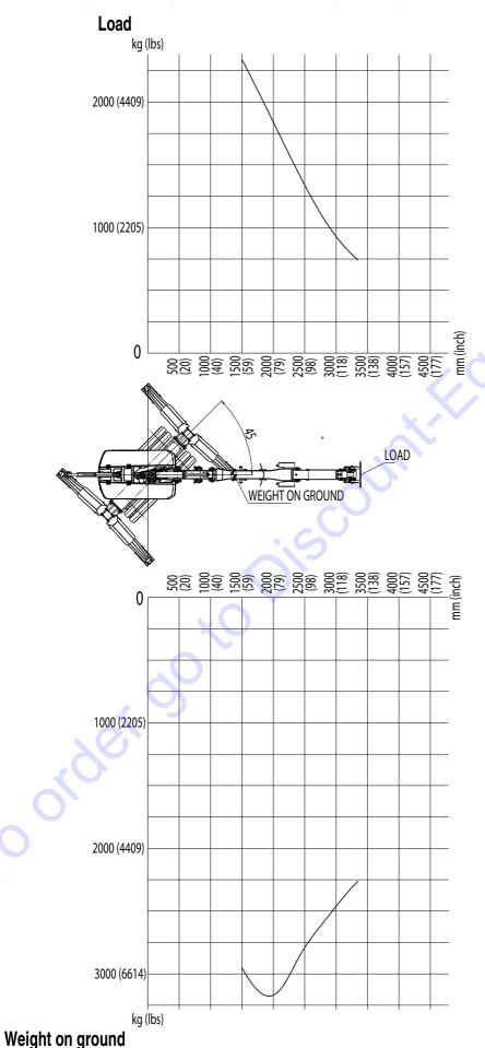
4. On tracks - forward DXR270 - weight on ground will appear on front end of both tracks.
