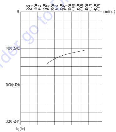
1. On outriggers – forward DXR310 - weight on ground will appear on two outriggers.
