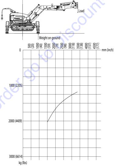
2. On outriggers – side DXR270 - weight on ground will appear on two outriggers.
