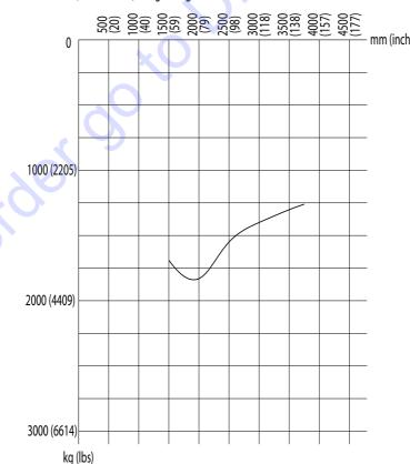
3. On outriggers – diagonal DXR300 - weight on ground will appear on single outrigger.
