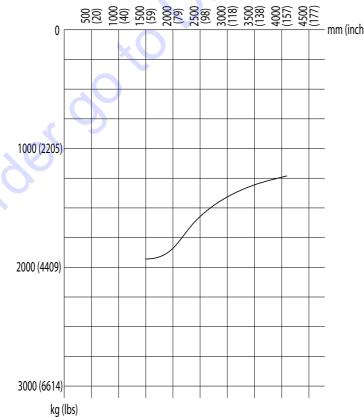
3. On outriggers – diagonal DXR310 - weight on ground will appear on single outrigger.
