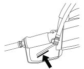
Press the switch lock and check that it returns to its home position when released.
