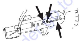
Unscrew the nuts and lift off the front belt guard.
