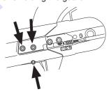
Take off the old belt and fit the new one. Fit the cutting arm to the machine and tension the belt with the adjuster screw. A new drive belt should be re-tensioned after running for about 30 minutes.
