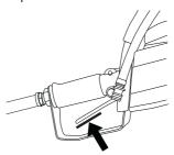
Press the switch lock and check that it returns to its home position when released.
