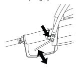
Start the machine, release the switch, and check that the machine and blade stop.
