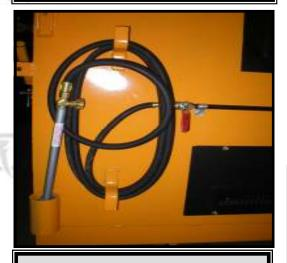
The KM 55 is equipped with a utility torch for heating the valve, tools, pour pots, etc.
