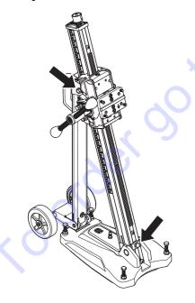
Loosen the locking screws for column tilt and set the desired drill angle. Tighten the locking screws. Use the feed lever. The column can be tilted 0-60°.
