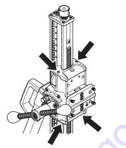
· Loosen set screws holding guide roller shafts.
