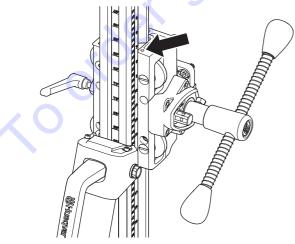
• Start with the top guide roller. Use a flat screwdriver and turn clockwise to guide the roller closer to the column.
