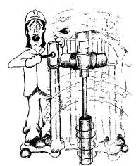
Water - Not too little and not too much-The right amount removes slurry and keeps the cut clean.
