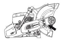
Rotate the bearing housing to opposite direction and reassemble the stop.
