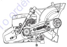
Fit the belt guards and tighten the nuts (A) finger tights. Wiggle the blade guard (E) up and down 3-5 times, and then tighten the nuts (A) with the combination spanner.
