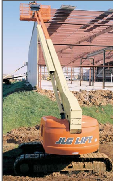
The 600 Crawler Series is equipped with all-steel tracks.
