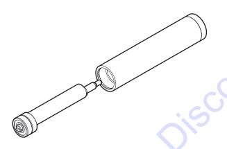
4. Press the two bearings out of the tube.
