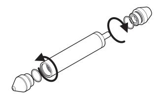
2. Loosen the square screw cap on the drive side by locking the eccentric. Use a screwdriver to lock the eccentric, place the screwdriver into the groove at the end with the end cap.
