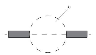
1. Remove the protective cap (C) to reach the carbon brushes (B). Use a large flat bladed screwdriver to remove the cap.
