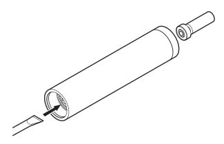
3. Locate the bearings and seals to be replaced. Pull out the eccentric together with the two bearings the vibrator tube. Pull out from the end with the end cap.
