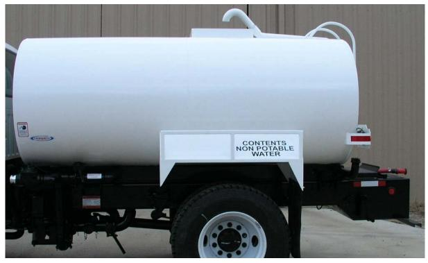
2000 Gallon Water Tank Mounted On Single Axle Truck
