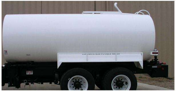
4000 Gallon Water Tank Mounted On Tandem Axle Truck
