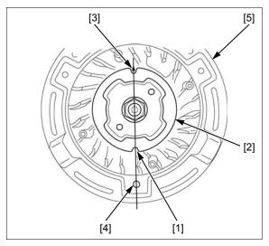
Insert a feeler gauge [1] between the valve adjust screw [2] and valve stem [3] to measure the valve clearance.
