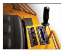
A 3-position switch directs the impact force to the front, rear or both drums, providing compaction where needed. The 4-in-1 control puts vibe on/off, direction, speed and braking at your fingertips.
