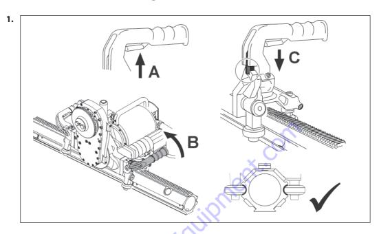
**2.** If the grips fail to engage or the wall saw sits too loosely on the guide rail: adjust the guide rollers.
