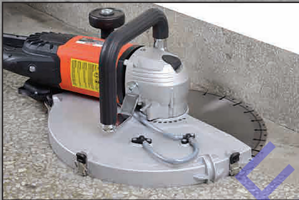
Removable guard side for flush cutting*
