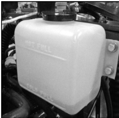
Coolant Recovery Tank – CC7574DK
