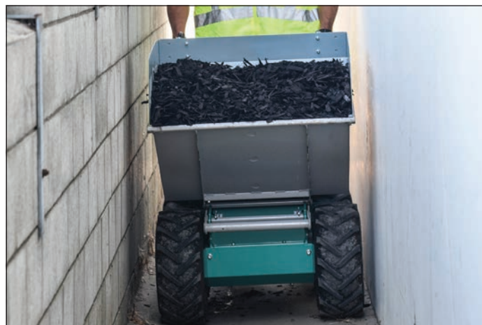
Optional 7 ft 3 clip-on tub — TT7 — allows access through narrow 32-inch passageways.
