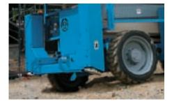
**OSCILLATING AXLE** Genie's oscillating axle automatically senses the terrain and adjusts the axle position based on ground conditions for maximum stability.
