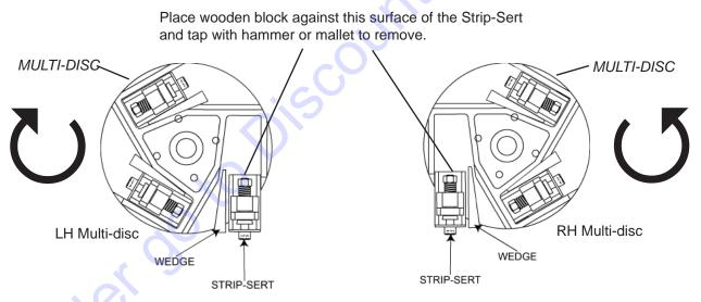
To remove an accessory, there are several different types, all are removed in the same manner, use a wooden block as explained in the above illustration. Never hammer directly on any accessory, damage to the self adjusting system will result and the accessory will have to be replaced.
