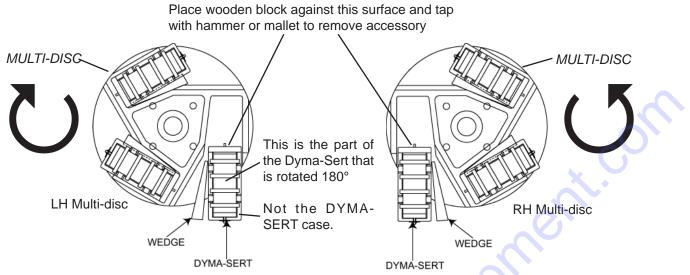
To install an accessory, there are several different types but all install in the same manner, use a brass rod or similar malleable material to drive the wooden wedge into place as shown in the above and below illustrations, note on which side of the accessory the wooden wedge is positioned (near center of disc). Never mix worn or used accessories with new ones. It will cause vibration and an uneven work surface. Replace accessories in complete sets, never mix sets.
