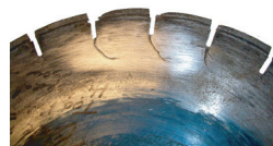
Cracked Segments And or Core Wrong Blade for job
