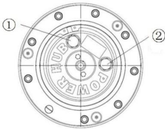
Figure 1-3 Traveling slowdown 1. Oil filler 2. Viewing port
