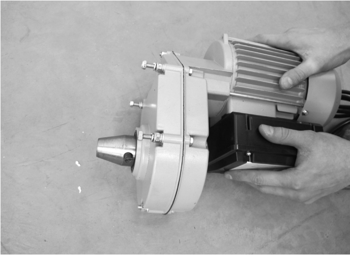
Remove nuts and washers from motor studs.
