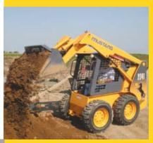
**Engineered to get more** work done in less time, the machines are designed with an SAE rated operating load of 1,050 lbs. for the 2026 and 1,350 lbs. for the 2041. An optional weight kit increases rated capacity by 125 lbs.
