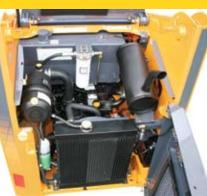
Rear engine cover and rear door open for easy engine/service access.
