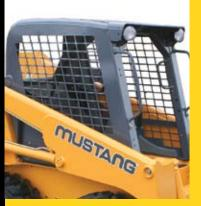
Mustang's ROPS/FOPS certified cab provides a protected and secure work environment for the operator. The ROPS/FOPS easily tilts up and out of the way for service access.
