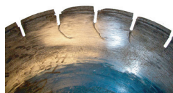
Cracked Segments and/or Core: Wrong blade for the job
