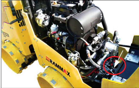
Fig. 9-29 Cable/connector Y9 under the hood
