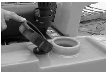
Figure 9. Checking Water Tank
