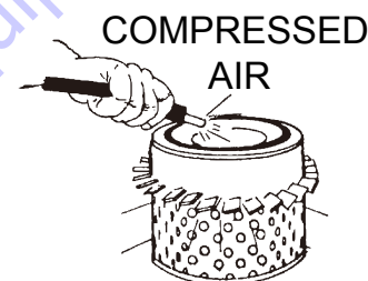
Figure 23. Cleaning Air Cleaner Element
