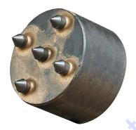
Use 5-Point bits for general purpose removal of concrete due to spalling, blistering, excess surface material, or in preparation of bonding new concrete overlays. Depth of removal is generally 1/4" or more and is dependent on the speed with which the unit is moved across the surface.
