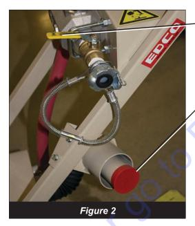
Position yourself behind machine and turn lever to run position and proceed to operate machine.
