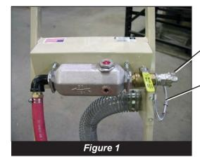
Connect air supply hose to connector on machine.
