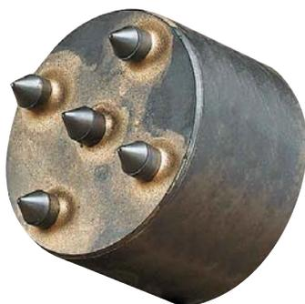
Use 5-Point bits for general purpose removal of concrete due to spalling, blistering, excess surface material, or in preparation of bonding new concrete overlays. Depth of removal is generally 1/4" or more and is dependent on the speed with which the unit is moved across the surface.
