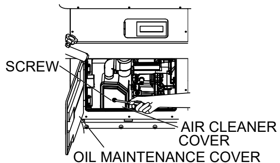
Figure 45. Removing Air Cleaner Cover
