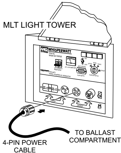
Figure 20. MLT Ballast 4-pin Power Cable
