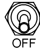
Figure 16. Manual-Off-On SW. (OFF Position)
