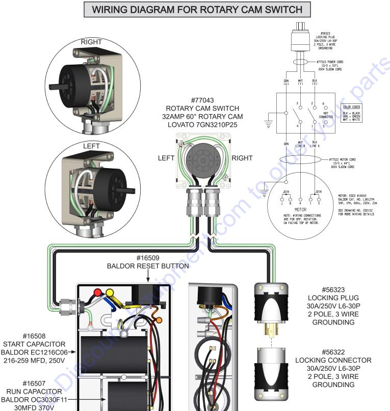
JUNCTION BOX DETAIL FROM: MOTOR: EDCO #16043 BALDOR CAT. NO. L3612TM 5HP, 1HP, 60Hz, 230V, 23A
