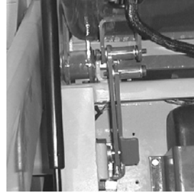
Figure 24 ROPS Lock Mechanism
