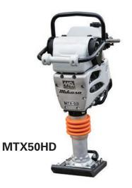
Weight Ibs (kg) - 129 (59) Shoe Width in (mm) - 10.4 (265) Engine Option - Honda GX100 Impact Force Ibs (kN) - 2,316 (10.3)
