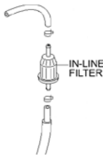
Figure 12. In-Line Fuel Filter
