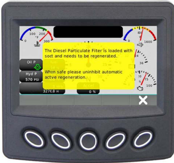
Figure 53 Yellow Regeneration Caution Single Screen Example
