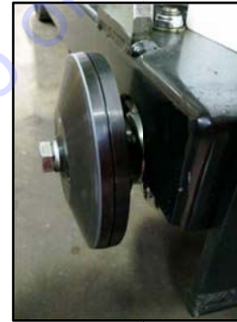
Figure 16: Blade Flanges Together
