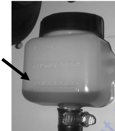
Figure 81 Expansion Tank Cold Line
