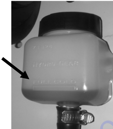
Figure 67 Expansion Tank Cold Line
