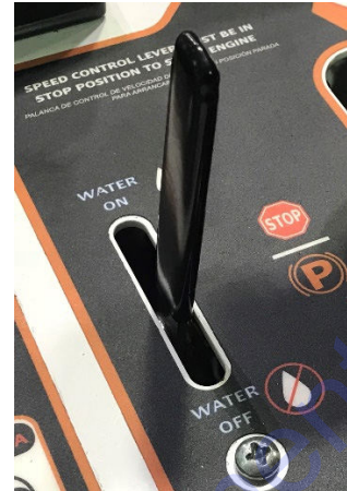
Water Control Valve
