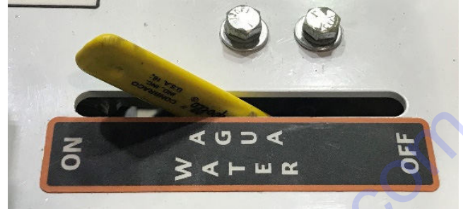
Water Valve - ON
