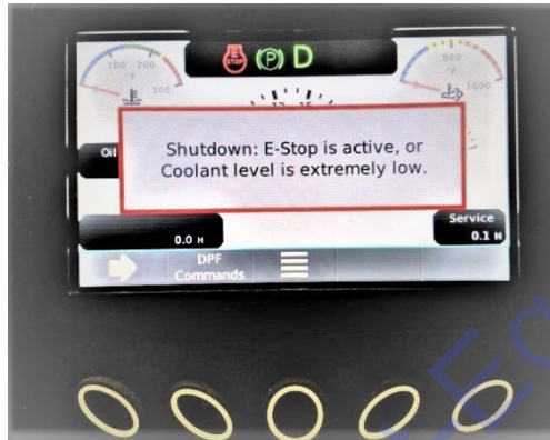
Main Gauge Screen with Emergency Shutdown Window
