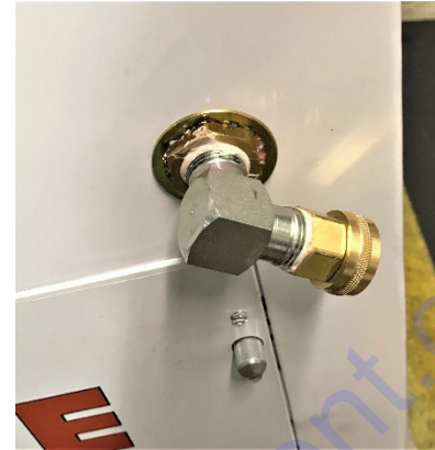
Water Supply Connection
