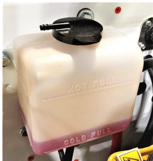
Coolant Recovery Tank
