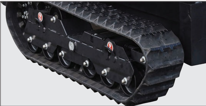
Aggressive tack pattern for use in soft soil to muddy site conditions.
