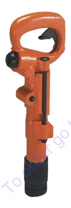
Weighing only 9 lbs, the APT Model 109 Rock Drill & Utility Drill is the lightest tool American Pneumatic makes. It is the ideal tool for drilling holes for anchor bolts as well as for small dowel hole drilling. The stop rotation feature easily converts the tool from a drilling machine to a percussion only tool.
