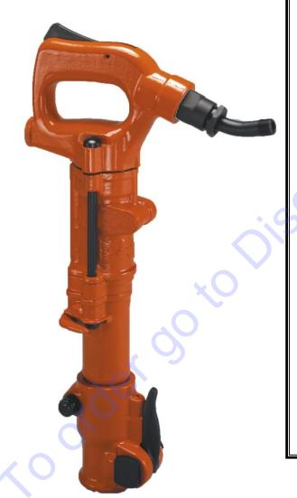
The APT Model 115 Rock Drill works as a drilling tool for drilling holes for anchor bolts and small dowel hole drilling. This versatile tool has a stop rotation feature that converts it from a drilling tool to a percussion tool. It is an ideal tool for light chipping in horizontal and overhead work.
