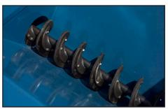
Patented Talet<sup>®</sup> auger with replaceable, composite polymer flighting, flexes to prevent binding. Provides superior flow control and efficiency. Auger can be run in two directions. Forward initiates flow of material – Reverse closes the flow valve and stops material discharge.
