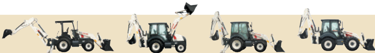
Four models available from 15,151 to 17,663 lbs. and standard dig depths of 14' 8" to 15' 11".
