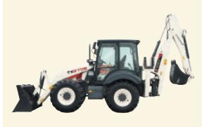
TEREX loader backhoes range from 86 to 94 hp, feature operating weights from 15,151 to 17,663 lbs., and provide standard digging depths from 14 ft. 8 in. to 15 ft. 11 in.
